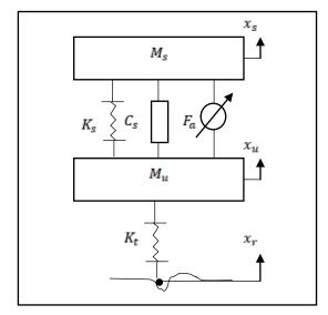
Fig. 1 Quarter vehicle model (Active suspension system)
